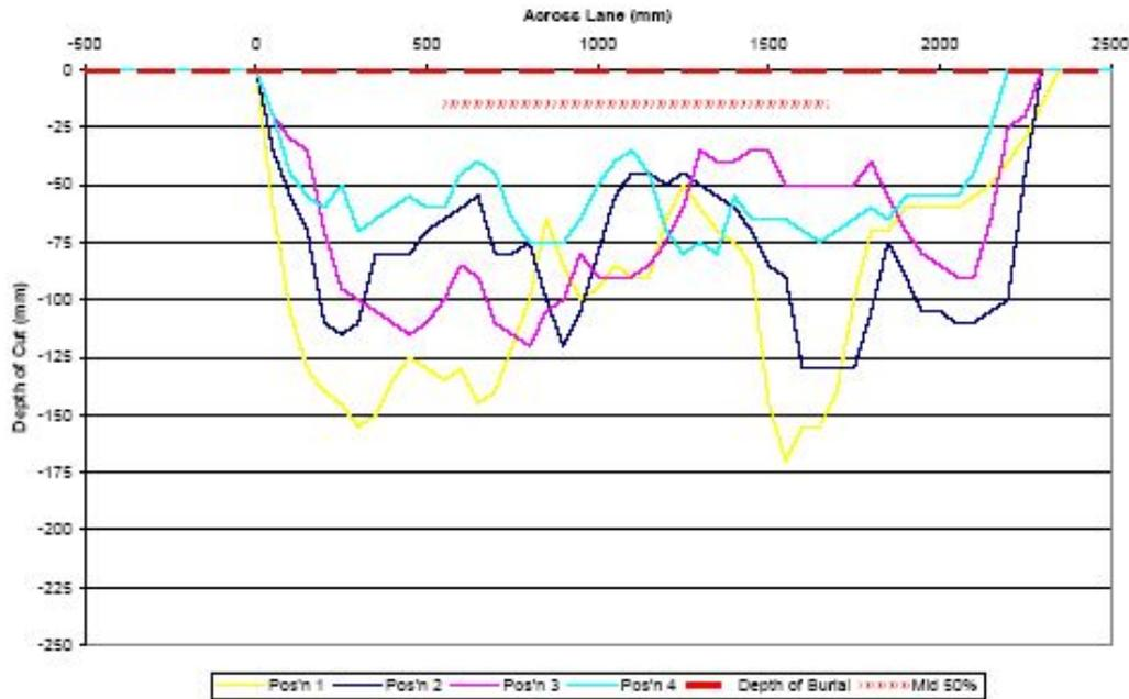
Figure 2: Ground penetration profiles determined using direct measurements. Ground penetration profiles were measured at 4 locations along the test lane.
